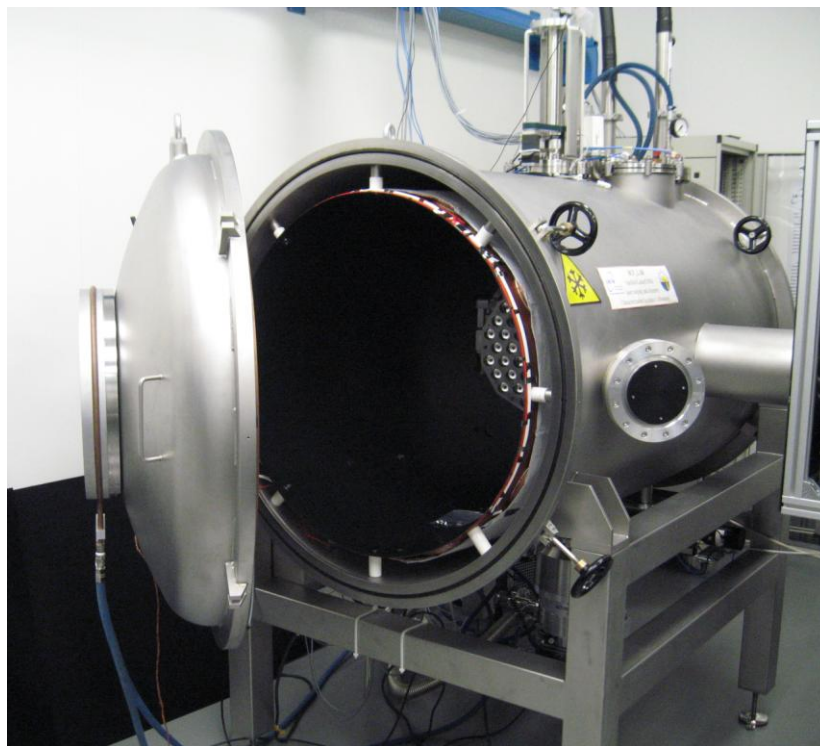
Figure 4. SCF-G cryostat with GNSS LRA installed prior to testing. The IR measurement port is shown on the right (Ge window hidden by a black cover)
